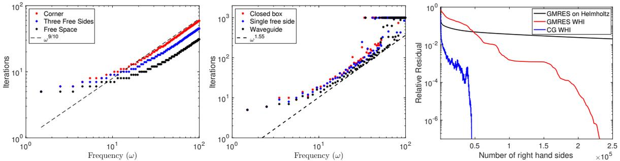
Fig. 4.6: To the left: number of iterations as a function of frequency to reduce the relative residual below  $10^{-7}$  for problems with no trapped waves. Middle: the same but for problems with trapped waves and for the interior problem. Both are with the GMRES accelerated WHI. To the right: Residuals for the GMRES accelerated WHI, the CG accelerated WHI and for GMRES solution of the directly discretized Helmholtz problem.
