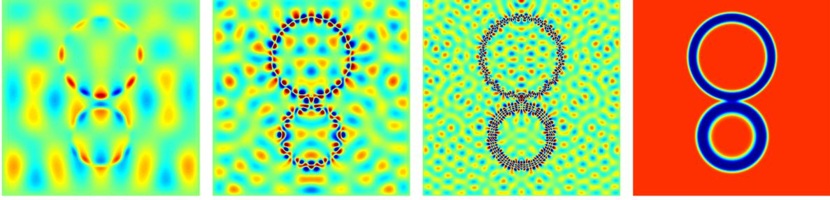
Fig. 4.12: Computation of three Helmholtz problems by one solve. The frequencies are  $\omega = 15, 30$  and  $60$ . The material model is also displayed, red is  $c^2 = 1$  and dark blue is  $c^2 = 0.1$ .
