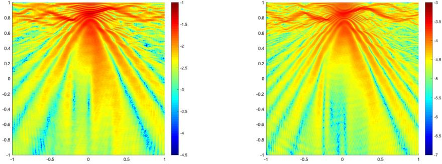
Fig. 4.14: Displayed is the base 10 logarithm of the magnitude of the Helmholtz solution ( $\log_{10} |u|$ ) caused by a point source near the surface for  $\omega = 200$  (left) and  $\omega = 300$  (right) at the slice  $x = 0.1$ .
