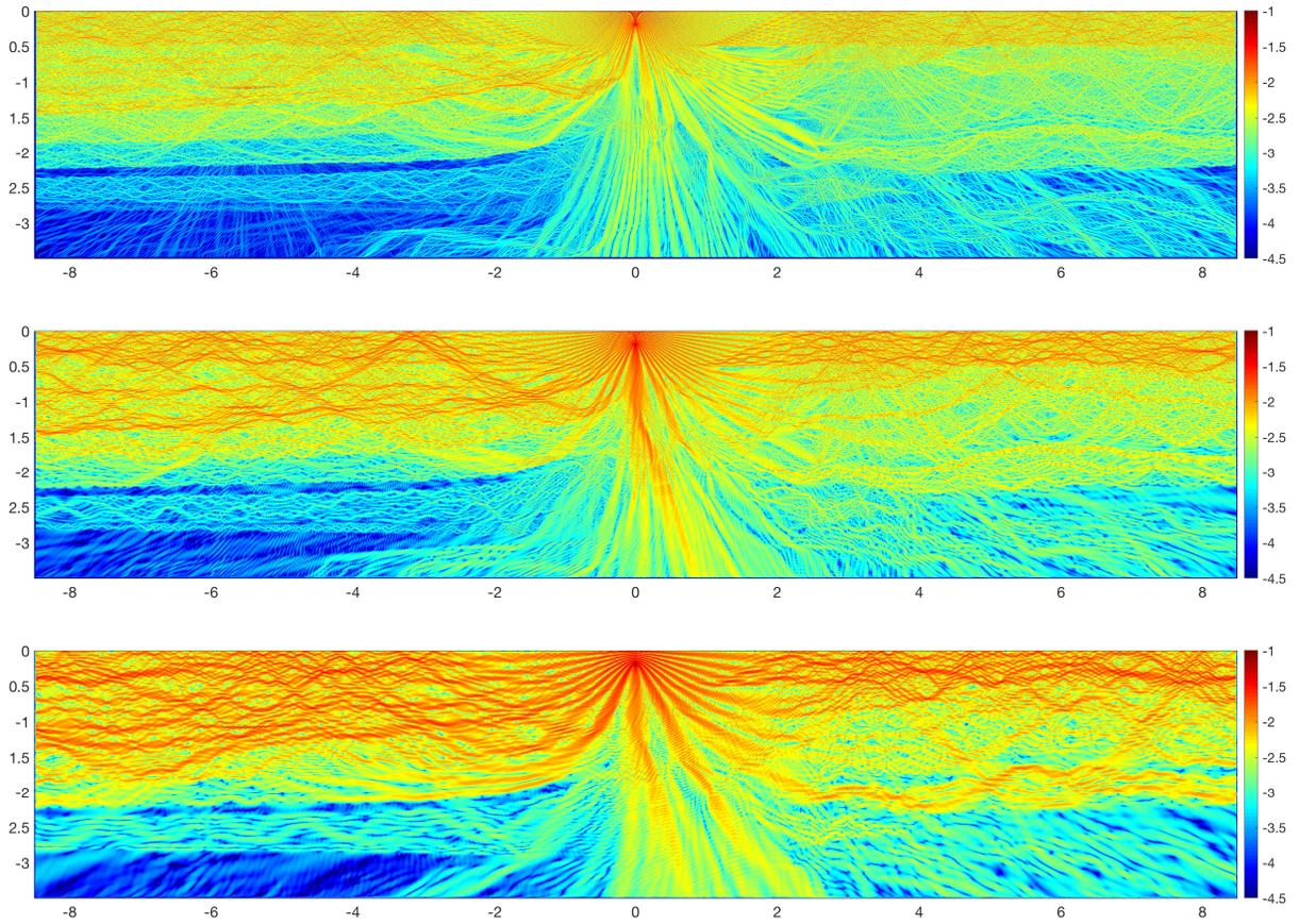
Fig. 4.10: Displayed is the base 10 logarithm of the magnitude of the Helmholtz solution ( $\log_{10} |u|$ ) caused by a point source near the surface. The results are, from top to bottom, for  $\omega = 800, 400$  and  $200$ .
