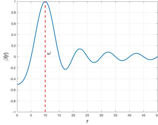
Fig. 2.1: The filter transfer function  $\beta$  for  $\omega = 10$ .
